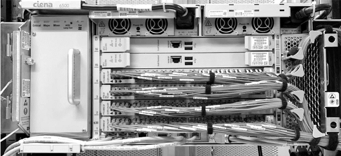
Use external fiber management drawers to store excess fiber cable. Fiber slack storage is not provided for fibers leaving the 6500 shelf.
