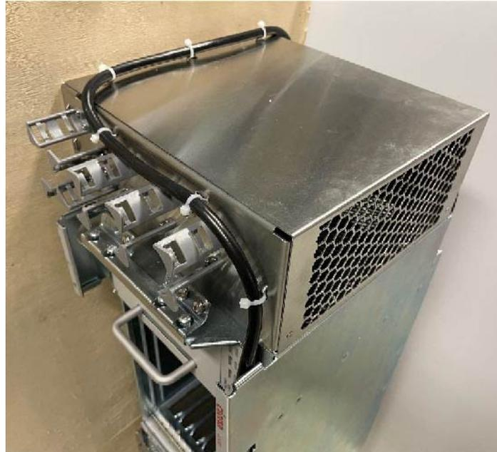
**Note:** Routing and securing to tie features shown is similar for DC power cables.
