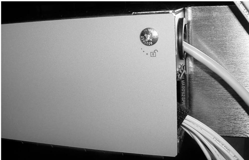
The internal fibers are already routed inside the OMX 16CH DWDM drawer.
