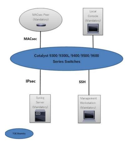
The TOE can be administered interactively using a CLI over a local console connection or remotely over SSH.
