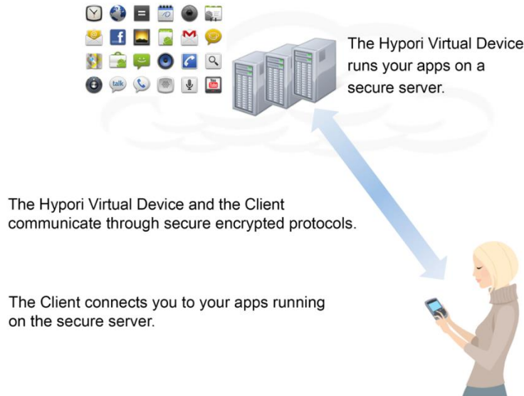
Figure 3 Hypori Halo Client Communication with a Hypori Virtual Device on a Hypori Server
